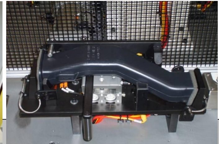
GMT901/902 DUCT BUBBLE CUT / PUNCH & PRESSURE TEST POKE YOKE MACHINE
